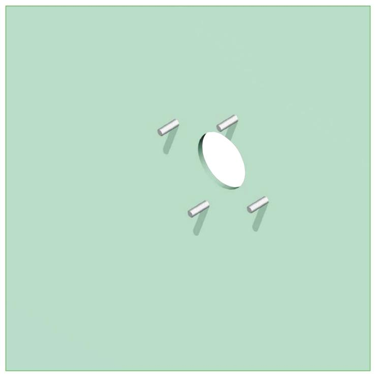
1) When DYNATITE<sup>®</sup> conduit sleeves for bolting are going to be used, a hole has to be cut in the partition to the size of the opening in the retainer flange of the DYNATITE<sup>®</sup> conduit sleeve. Threaded ends have to be welded to the partition in accordance with the hole configuration of the flange of the conduit sleeve. In case of application against concrete walls, stainless steel anchor bolts should be used.
