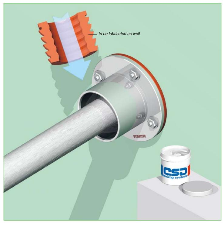
5) The inside surfaces of both segments of the DYNATITE<sup>®</sup> sealing plug are then lubricated with CSD<sup>®</sup> lubricant. Also the flat contact surfaces of the plug halves should be lubricated to enable equal insertion in the conduit sleeve. CSD<sup>®</sup> lubricant is acid free.
