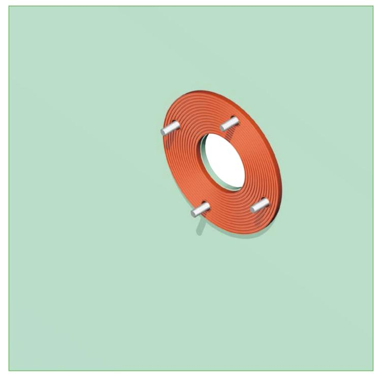
2) A fitting NOFIRNO<sup>®</sup> gasket is placed over the threaded ends against the partition.
