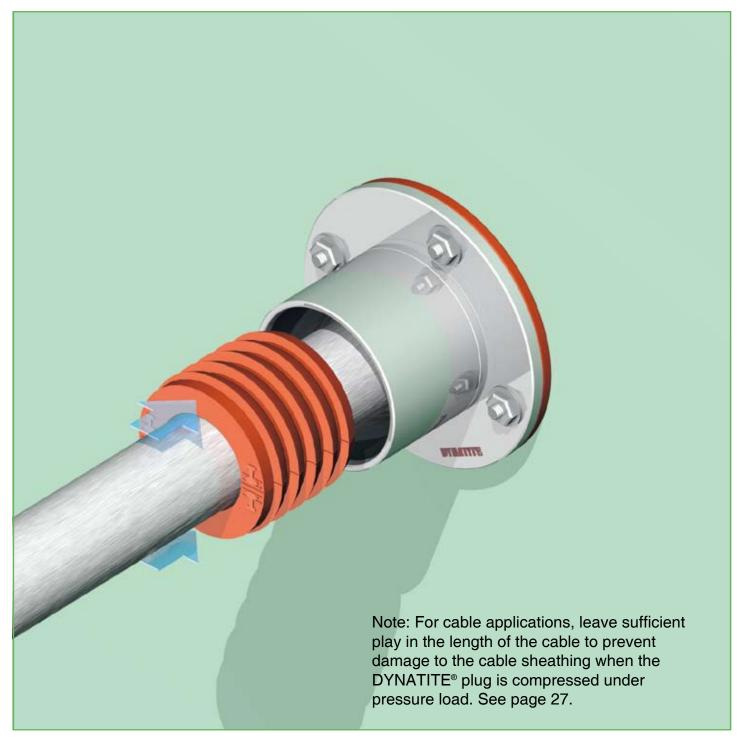
7) Both segments of the DYNATITE<sup>®</sup> sealing plug are placed around the ducted pipe/ cable, then pushed into the conduit sleeve as far as the first serration. The first serration is smaller than the other serrations to make this procedure very easy. Both halves are then pushed by hand evenly, further into the DYNATITE<sup>®</sup> conduit sleeve. The inlet of the DYNATITE<sup>®</sup> conduit sleeve is rounded off to avoid any damages to the plug during insertion.
