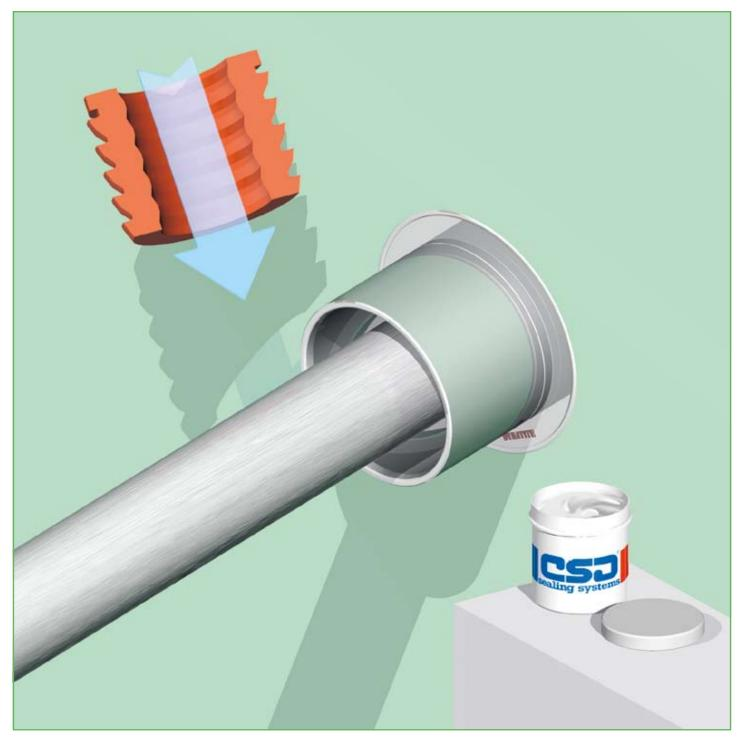
3) The inside surfaces of both segments of the DYNATITE<sup>®</sup> sealing plug are then lubricated with CSD<sup>®</sup> lubricant. Also the flat contact surfaces of the plug halves should be lubricated to enable equal insertion in the conduit sleeve. CSD<sup>®</sup> lubricant is acid free.
