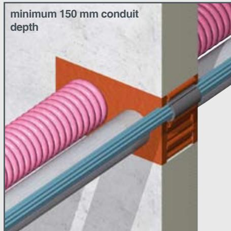
RISE<sup>®</sup>/NOFIRNO<sup>®</sup> cable penetrations have been tested with heavy conductor cables. The length of the conduit could be further minimized without the use of extra insulation by the thermally insulating properties of the NOFIRNO<sup>®</sup> filling. With 150 mm conduit depth already a fire classification E120/EI120 has been achieved. With increased conduit depths the rating will be higher.
