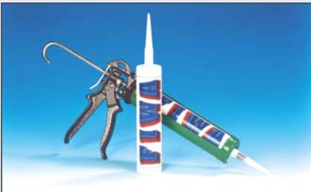
For ease of application of very high viscosity sealants, we have selected a powerful manual applicator with a 26 : 1 trigger leverage. This means much easier dispensing and reduced fatigue. The applicator is equipped with the so-called Wear Compensating Device, which automatically removes free-play in the trigger to provide instant rod drive immediately when the trigger is pulled. Less full trigger strokes required to empty a cartridge. Extended working life of the applicator.
