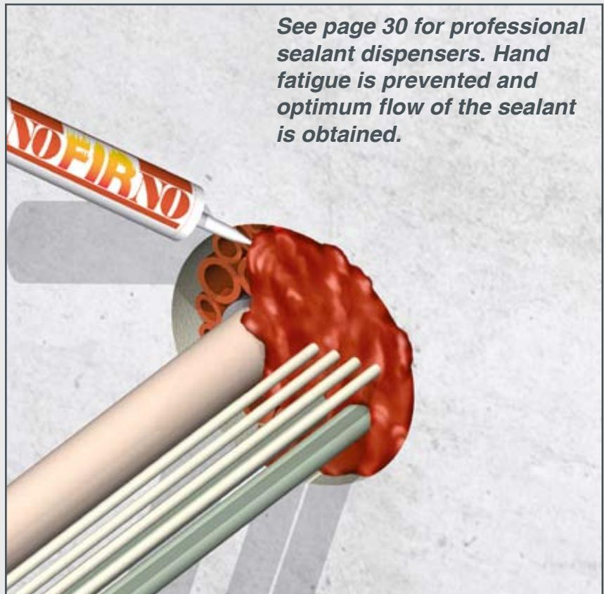
*See page 30 for professional sealant dispensers. Hand fatigue is prevented and optimum flow of the sealant is obtained.*
