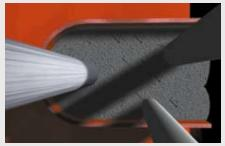
Generally, rubbers used for multi-cable transit systems are made of a more or less self-extinguishing compound. The drawback, however, is that these rubbers will start charring under heat and slowly but surely will shrink due to the loss of the water content in the rubber. *Not with RISE* <sup>®</sup>! The rubber starts vulcanizing when exposed to heat, forming a solid rubber mass inside the penetration and an expanding char on all exposed surfaces.
