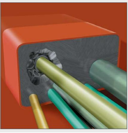
For the EMC protection of cable penetrations entering shielded areas, an electrically conductive sealant/flexible rubber is developed for the RISE® multi-cable penetrations type EMC. Tests carried out in our laboratories have shown that the electrical resistance from braiding to mass is about 1-2 ohm.
