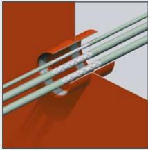
2) Remove the cable sheathing over a length that is 40 mm shorter than the length of the penetration, in such a way that the front face of the exposed braiding is situated about 20 mm inside the conduit at both sides.
