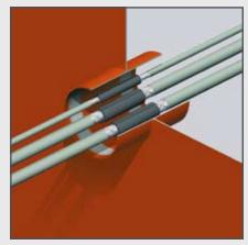
3) RISE® sleeves 120 mm shorter in length than the penetration are then fitted around the ducted cables and pushed into the penetration. The exposed braiding should extend 40 mm outside the sleeves.
