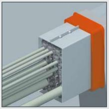
The flanges are 10 mm high, corresponding with the wall thickness of the block system transits. This enables the EXTEND-A-FRAMES to fit in multi-transit units without any problems. The EXTEND-A-FRAME, positioned in the transit frame, leaves 20 mm free at the back of the transit frame for the bonding of the FIWA® sealant to that transit frame. This is necessary to obtain a tight seal. Place a RISE® insert sleeve around each cable. Any empty space is filled with RISE® filler sleeves.
