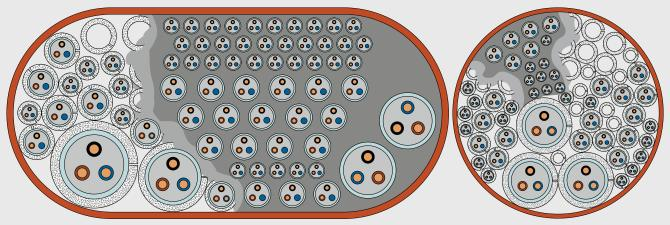
RISE® is designed to duct the maximum allowable filling rate of 40% as defined in the IMO Res. A.754(18).
