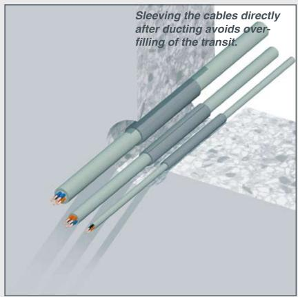
3) The remaining free space in the conduit is filled with RISE® filler sleeves type 27/19 and 18/12.
