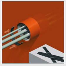
6) Then apply layers of CONDUCTON® flexible rubber strips 40 mm wide against the inside wall of the penetration.
