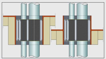
The easiest way to pass a deck test is to place the transit totally above deck. Worst case for deck penetrations is to place the transits totally below deck. And that is exactly the way the penetrations generally are installed! Cable penetrations should be applied as tested. This means that penetrations tested only above deck should not be placed totally below deck. RISE® multi-cable penetrations are tested "worst case" and can be welded in above, below, midway.
