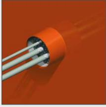
5) Push the insert/filler sleeves into the penetration in such a way as to leave about 60 mm free space at both sides. Take care that the exposed braiding extends 40 mm outside the sleeves at each side.
