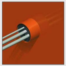
7) Pack the free space inside the penetration with lengths of strip.
