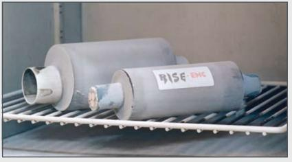
What will the performance of a fire safe multi-cable penetration be after years of service? *Remember that safety is at stake here.* This is the reason why the RISE® system has been artificially aged up to 50 years, after which the expanding properties of the rubber and the sealant were compared with new material. Only minor changes were noted! Temperature cycle on the RISE® system from -40 °C to ambient to +120 °C, and back, showed that the adhesion of FIWA® holds the system tight!
