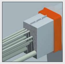
Center the RISE® sleeves within the conduit so as to leave 20 mm free space at the front and the back of the transit. A 20 mm layer of FIWA® sealant is applied at both sides of the transit. Refer to the step by step installation instructions for RISE® multi-cable penetrations for final finishing of the transit.
