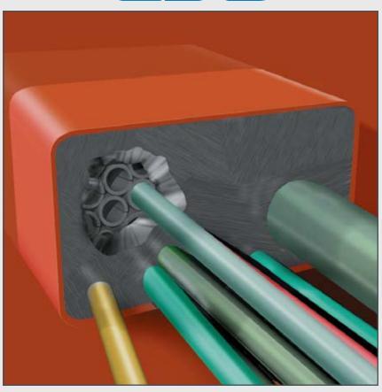
If the empty filler sleeves are not fitting to the size of the cable to be ducted, a number of these insert sleeves must be removed from the penetration. Install a fitting insert sleeve (with some filler sleeves if necessary) in the open space in the penetration.
