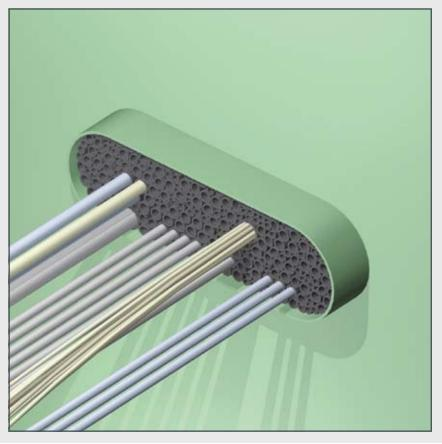
The RISE® sealing system allows cables to be ducted through conduit openings in a bent, curved or oblique way without any adverse impact on sealing performance. Due to the fact that RISE® is an adhesive system, only proper contact surfaces are needed to obtain tightness. Sufficient cable separation is a must to enable the FIWA® sealant to be applied in between the cable set.
