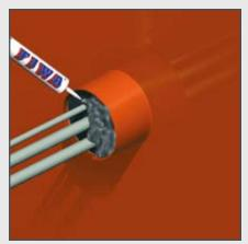
10) At both sides of the penetration about 20 mm free space should be present to enable the application of the FIWA® fire safe, water tight sealing compound. First clean the inside wall of the penetration very thoroughly.
