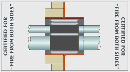
Section A.IV/2.2.1 of IMO Res. A.754(18) states "A bulkhead which includes the cable transit should be constructed in accordance with 2.1.1 of the recommendation and should be insulated to class A-60 on the stiffened side, which should be the face which is not exposed to the heating conditions of the test." Systems tested with insulation at the exposed side have a limitation in the application. The bulkhead must then be totally insulated at both sides! This is not the case with RISE®.
