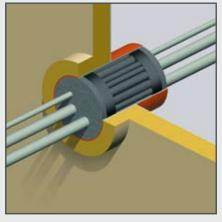
14) For A-class penetrations the conduit sleeve/frame needs to be insulated only at the insulated side of the bulkhead or at the lower side of the deck.
