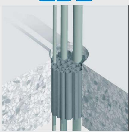
2a) Pull a set of bundled cables through the conduit and place a RISE® insert sleeve around the cable.
