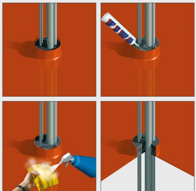
RISE® multi-cable transits are also used for water or gas tight conduits in buildings and constructions. When fire rating is not a requirement, the conduit length for only water and gas tight conduits can be reduced substantially. With a view on ease of installation, it is advisable not to use insert and filler sleeves with a length shorter than 60 mm. We always recommend to apply a layer of FIWA® sealant about 20 mm thick on both sides of the penetration.
