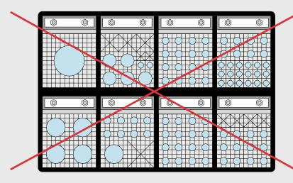
Since the cables can be ducted in random order through the conduit frame or sleeve it is not necessary to create lay-outs for the installers to be sure that the cables are ducted at the right spot in the conduit. We have a software program available for calculating the size of the conduit opening and the amount of insert sleeves and sealant for each RISE® penetration. All penetrations can be put in a database to calculate the total amount for a project (see page 35). Could it be easier?
