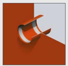
1) At the place where the CONDUCTON® flexible compound is to be applied, the penetration should be bare steel without primer and thorougly cleaned to ensure effective connection to earth.
