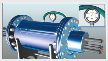
Due to the high bonding strength and flexibility of the FIWA® sealant, the penetrations could be subjected to certified pressures up to 2.5 bar (35 Psi) without any leakage. Where rubber parts have to be strongly compressed to obtain water tightness, they will soon show permanent deformation. Also, the cable sheathings are exposed to this heavy load and will creep. This is not the case with RISE®. *Tight stays tight, with no compressive forces on the cables! CERTIFIED.*
