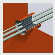
4) The remaining space inside the penetration is then packed with RISE® filler sleeves. Push the filler sleeves into the penetration in the same way as the sleeves fitted around the cables. Make sure that the sleeves fit tightly.
