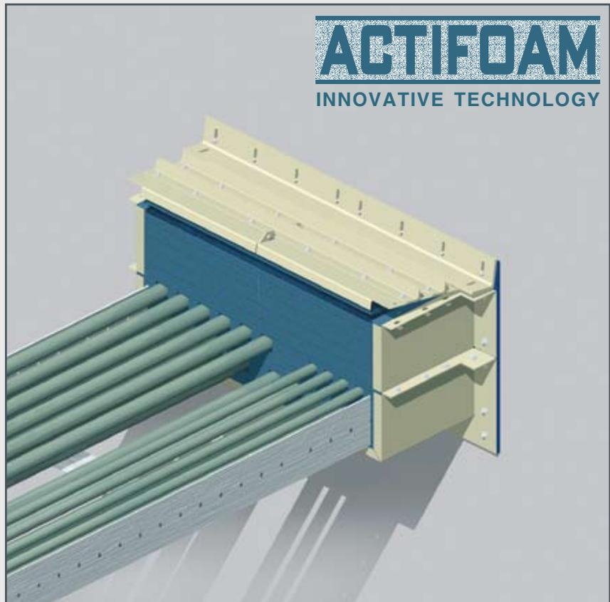
23) The cable(s) can be ducted and separated in the way as described before. Then the firestop can be refilled with the removed ACTIFOAM® filling and the cover plate can be fixed again on the casing.
