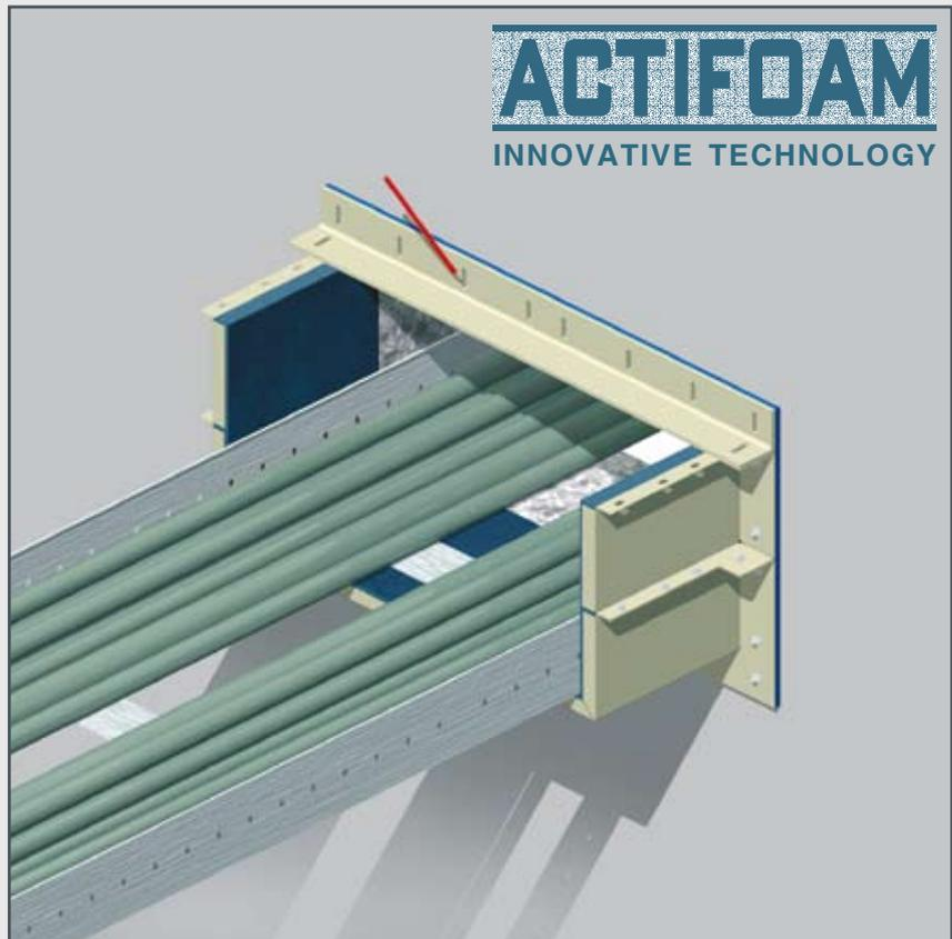
8) After drilling, position the anchoring bolts and the attachment bracket. Do not tighten the bracket firmly, in order to facilitate insertion of the top layer of rubber pads later during installation.
