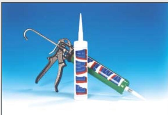
For ease of application of very high viscosity sealants, we have selected a powerful manual applicator with a 26 : 1 trigger leverage. This means much easier dispensing and reduced fatigue. The applicator is equipped with the so-called Wear Compensating Device, which automatically removes free-play in the trigger to provide instant rod drive immediately when the trigger is pulled. Less full trigger strokes required to empty a cartridge. Extended working life of the applicator.
