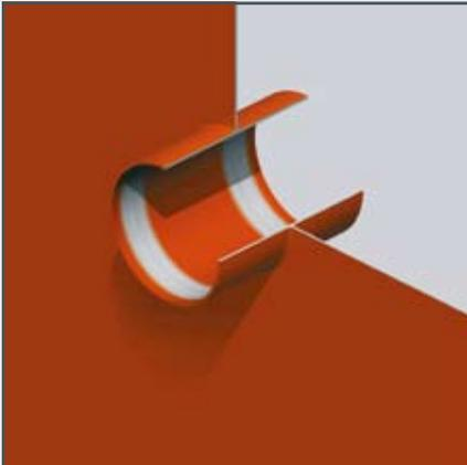
1) At the place where the CONDUCTON<sup>®</sup> flexible compound is to be applied, the penetration should be bare steel without primer and thoroughly cleaned to ensure effective connection to earth.
