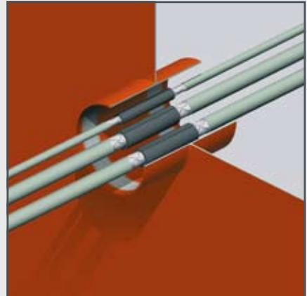
3) RISE<sup>®</sup> sleeves 120 mm shorter in length than the penetration are then fitted around the ducted cables and pushed into the penetration. The exposed braiding should extend 40 mm outside the sleeves.
