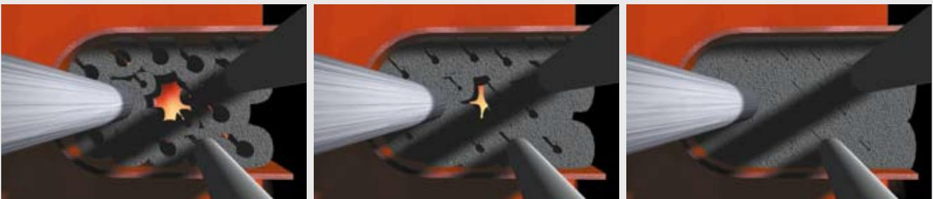
Generally, rubbers used for multi-cable transit systems are made of a more or less self-extinguishing compound. The drawback, however, is that these rubbers will start charring under heat and slowly but surely will shrink due to the loss of the water content in the rubber. **Not with RISE<sup>®</sup>!**
