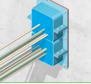
17) After smoothing is finished, a last check should be taken to ensure sealant is applied in between the cables, especially in penetrations with larger amounts of cables. For adding cables see page 29.
