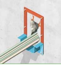
5) The split flanged frame is disassembled, and the lower part secured finger-tight against the wall. Both the CSD<sup>®</sup> frames and NOFIRNO<sup>®</sup> gaskets have oval holes for ease of adjustment.
