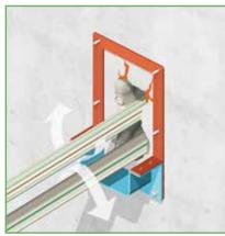
7) If utilizing multi-bay frames, separate the cables and place them in the bay where watertight sealing is most easiest. This may depend on the play in the cable set.
