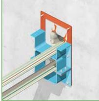
8) Position the intermediate element of the frame over the anchor bolts against the wall, and then fix the element to the previously positioned frame. Secure the intermediate element finger-tight against the wall.
