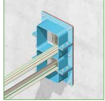
9) In the same way, place the upper part on the intermediate part. Tighten the bolts on the connector flanges. Note: no excessive forces needed. Finally, all the nuts on the anchoring bolts should be firmly tightened.
