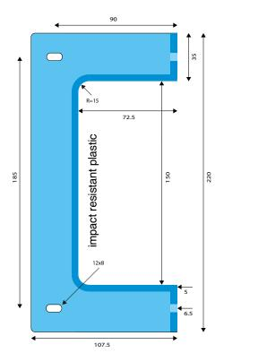
NOFIRNO<sup>®</sup> gaskets: top: side part of single bay frames (two pieces for each frame). middle: extension gasket for multi-bay frames (one or more sets, top-bottom, to be used. bottom: side part for multi-bay frames (two pieces for each frame).
