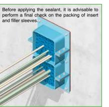
11) The remaining free space in the conduit is filled with RISWAT<sup>®</sup> filler sleeves type 27/10 and 18/12. The whole set of insert and filler sleeves should fit tightly into the conduit to provide sufficient mechanical stability.
