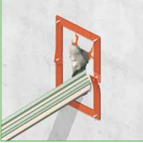
4) After drilling the attachment holes and positioning the anchoring bolts, place the NOFIRNO<sup>®</sup> gasket parts over the anchoring bolts against the wall.
