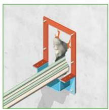
6) Place the NOFIRNO<sup>®</sup> gaskets on the connector flanges of the CSD<sup>®</sup> split flanged frame.
