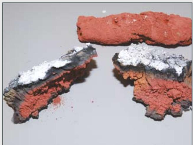
**RISE®/NOFIRNO® filler sleeves are made of NOFIRNO® rubber which will not be consumed in fire conditions. From the way of surface charring and the rubber residues inside the product, it can easily be determined whether or not NOFIRNO® has been used.**
