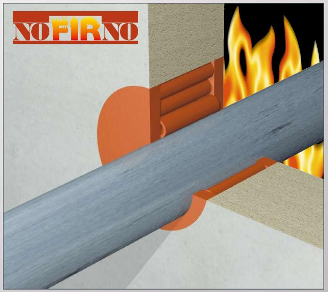
SUCCESSFULLY TESTED ACCORDING TO EN 1366-3:2004; FIRE RESISTANCE E190/E1120 ACCORDING TO EN 13501-2:2003 CERTIFICATES 2007-EFECTIS-R0763-64
