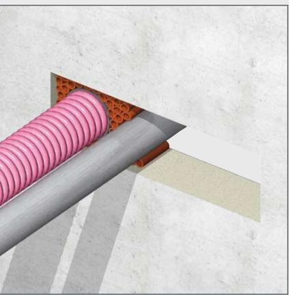
5) Bundled cable sets are allowed in the RISE<sup>®</sup>/NOFIRNO<sup>®</sup> multi-all-mix sealing system, using only one RISE<sup>®</sup> insert sleeve. See for details the approved installation drawings.
