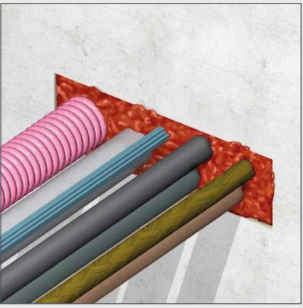
15) To smooth the surface of the FIWA<sup>®</sup> sealant layer, a cloth is sprayed with water. This prevents the sealant from sticking to the cloth. Note: do not use soapwater!
