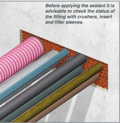
13) A 20 mm thick layer of NOFIRNO<sup>®</sup> sealant is applied at each side of the conduit. Clean and dry the conduit opening and the cables thoroughly and remove any dirt, rust or oil residues before applying the sealant.
