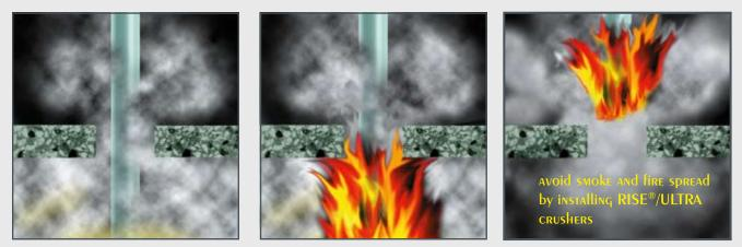
Based on the CRUSHER<sup>®</sup> technology it is now possible to make fire stop penetrations for plastic pipes just by inserting a single RISE<sup>®</sup>/ULTRA crusher into the conduit opening. The RISE<sup>®</sup>/ULTRA crusher trapped air to expand rather fast. In this way compression of the plastic pipe starts already at an early stage of the fire. The unique RISE<sup>®</sup>/ULTRA crusher allows for smallest conduit openings. For oversized
