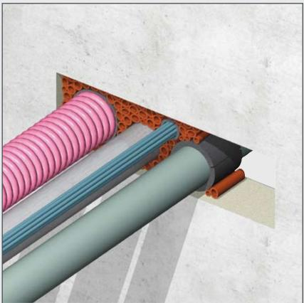
9) The system allows also for insulated chilled water lines without interrupting the insulation and multibeverage lines. A RISE<sup>®</sup>/ULTRA crusher or wrap is placed around the insulation and inserted into the penetration.
