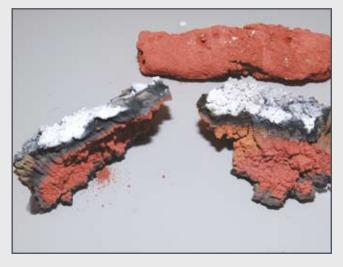
RISE<sup>®</sup>/NOFIRNO<sup>®</sup> filler sleeves are made of NOFIRNO<sup>®</sup> rubber which will not be consumed in fire conditions. From the way of surface charring and the rubber residues inside the product, it can easily be determined whether or not NOFIRNO<sup>®</sup> has been used.
