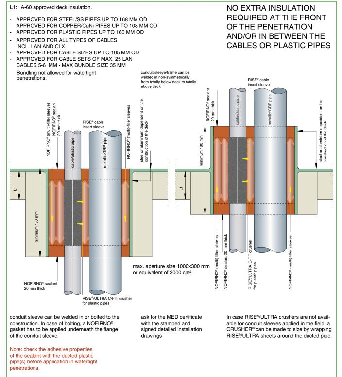
Specifications for A-class according to EC (MED) certificate MED-B-5068 issued by Det Norske Veritas. Drawings N0015E, N0016E and N0017E A0-A60 MULTI-ALL-MIX® PIPE/ CABLE TRANSIT
