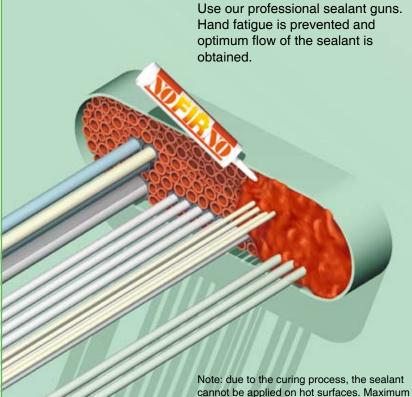
6) The conduit should be overfilled with NOFIRNO® sealant, because some sealant will be pushed between and into the empty filler sleeves during further finishing.
