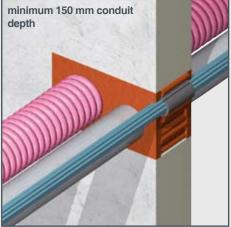
RISE®/NOFIRNO® cable penetrations have been tested with heavy conductor cables. The length of the conduit could be further minimized without the use of extra insulation by the thermally insulating properties of the NOFIRNO® filling. With 150 mm conduit depth already a fire classification E120/El120 has been achieved. With increased conduit depths the rating will be higher.
