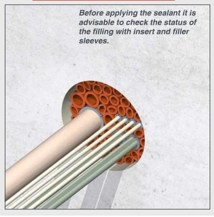
5) A 20 mm thick layer of NOFIRNO® sealant is applied at each side of the conduit. Clean and dry the conduit opening and the cables thoroughly and remove any dirt, rust or oil residues before applying the sealant.
