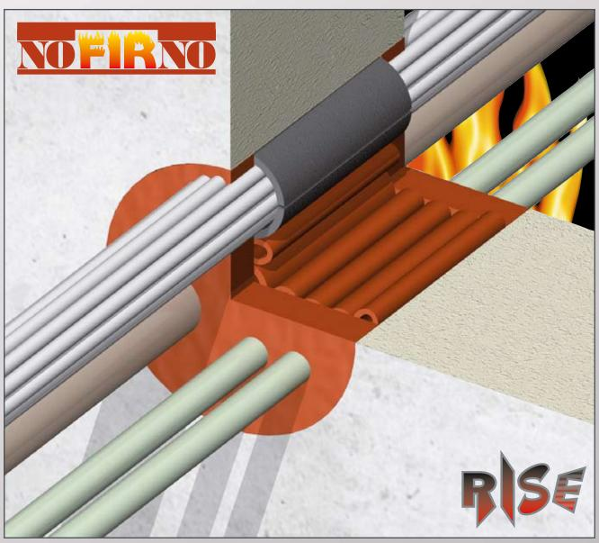
SUCCESSFULLY TESTED ACCORDING TO EN 1366-3:2004; FIRE RESISTANCE EI90/EI120 ACCORDING TO EN 13501-2:2003 CERTIFICATES 2008-EFECTIS-R0633-36
