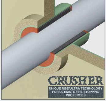
plastic pipe) transits. RISE®/ULTRA crushers have also been tested according to EN1366-3:2004 for a fire rating of two hours and lately in-house for a four hour fire rating.
